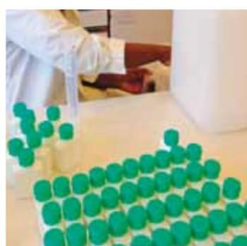
7. Immediately divide the solution into its final containers (e.g. 500 or 100 ml plastic bottles), and place the bottles in quarantine for 72 hours before use. This allows time for any spores present in the alcohol or the new/reused bottles to be destroyed.
