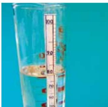
2. Post-production analysis is mandatory if either ethanol or an isopropanol solution is used. Use the alcohol meter to control the alcohol concentration of the final use solution. The accepted limits should be fixed to  $\pm 5\%$  of the target concentration (75%–85% for ethanol).
